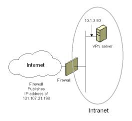
Figure 6 The single-adapter VPN server configuration
