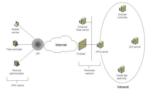
Figure 2 Components of Windows 2000 remote access VPNs
