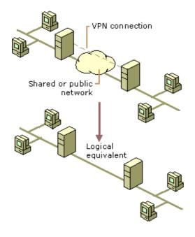
Figure 1 The logical equivalent of VPN connections
