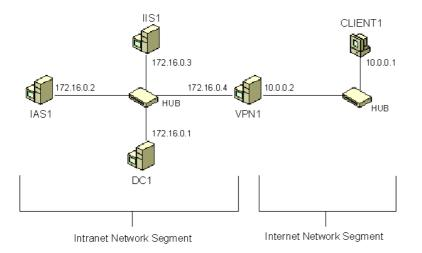
Figure 7. Configuration of the VPN test lab
